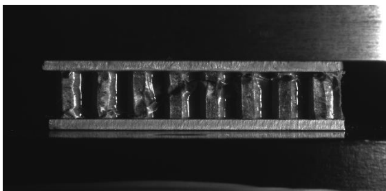
Figure 1: Experimental crushing of Nomex® honeycomb
